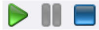
Figure 3.17: The green play symbol indicates that the process is currently in a breakpoint and can continue being executed if pressed.
