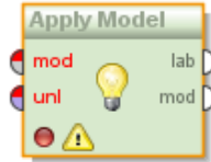
Figure 2.13: An operator can be connected via its input ports (left) and output ports (right).
