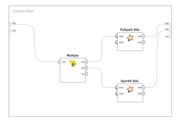
Figure 7.1: Tutorial process 'Running SparkSQL using the Python and R Spark API'.
